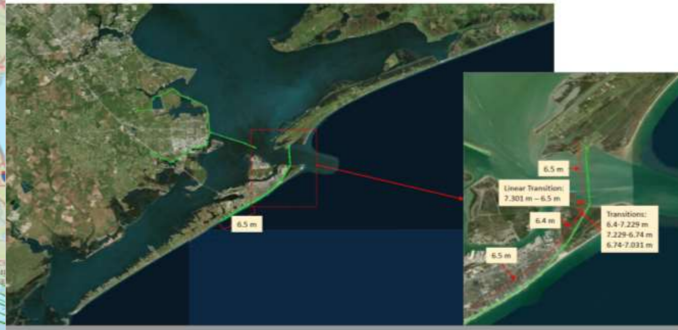
3) Gate at Bolivar, beach dune system, and a ring levee on the backside of Galveston Island
