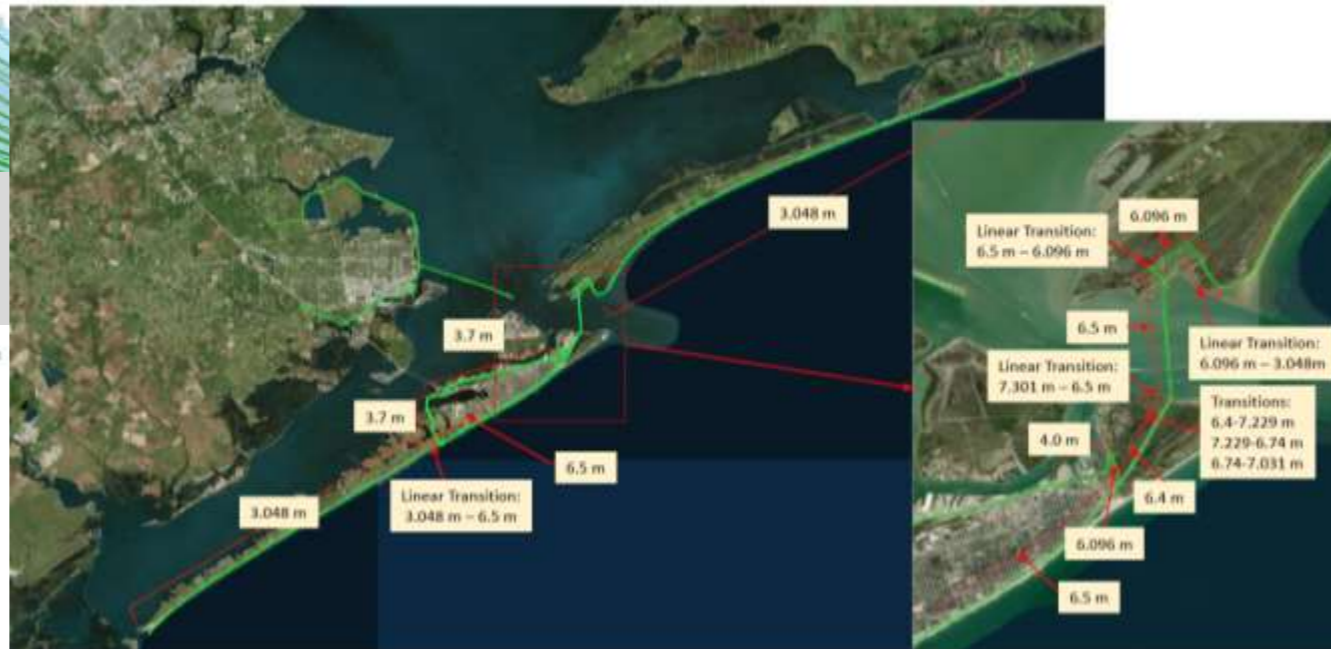
3) Gate at Bolivar, beach dune system, and a ring levee on the backside of Galveston Island
