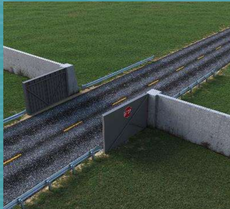
Example road/rail closure (open)
